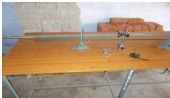
Fig. 1. Deflection test of simply supported beam
