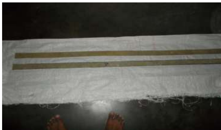
Fig. 2. Deflection test of simply supported beam showing the specimens of general Purpose resin (Polyester) and epoxy resin
