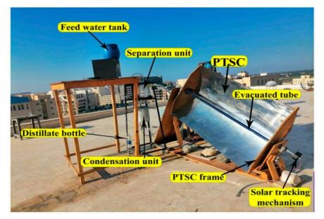
Fig 1. Photograph of test-rig.
