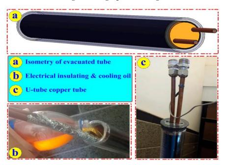
Fig. 2 PTSC Evacuated pipe
