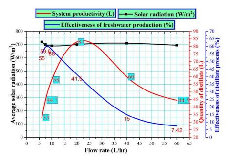
Fig. 6 system performance of different water flow rates
