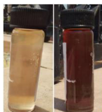
Fig.2. Reaction mixture (soybean seeds extract and silver nitrate solution) before (left) and after (right) solar exposure
